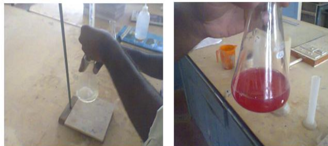
Figure 5.3 Titration of acid solution with 1N NaOH base solution
