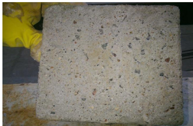
Figure 6.3 Specimen of normal SCC immersed in 5% H_2SO_4
