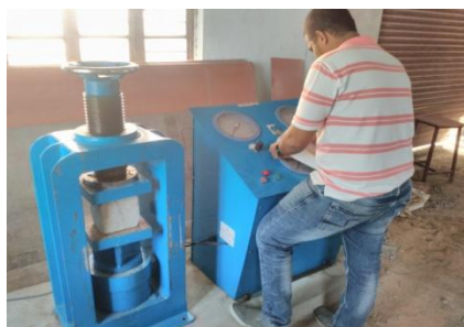
Figure 5.1 CTM where cubes are tested for compressive strength
