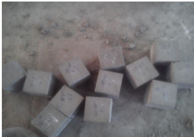
Figure 4.1 Cubes demoulded after 24hrs of casting
