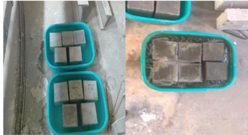
Figure 5.2 cubes immersed in 5% H 2 SO 4 and 5% HCl
